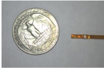
Figure 2.2 qOCE probe compared to a US quarter.
